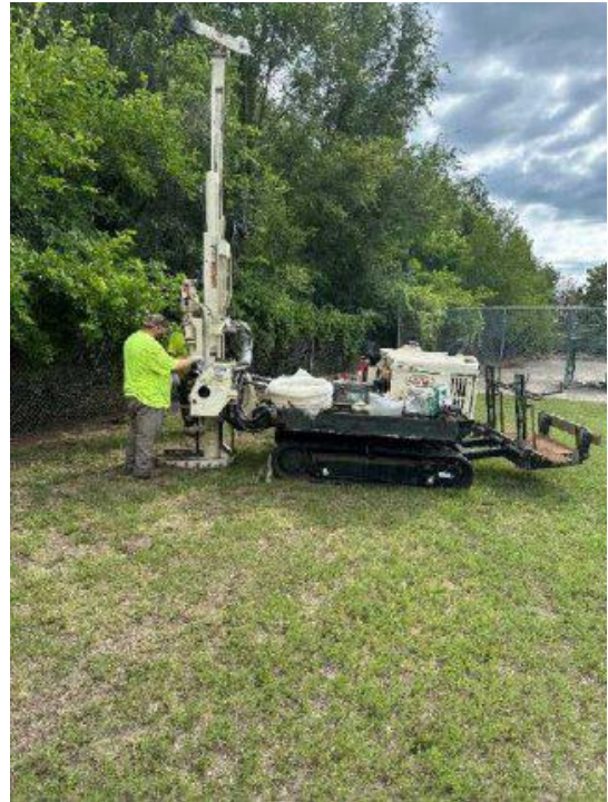
This photograph shows direct push technology (DPT) use to collect groundwater samples at B-2.
